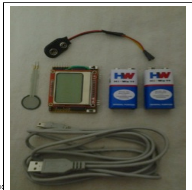
Image 1- dismantled system showing the component parts (top) battery connector (middle row L to R) sensor, device, batteries
